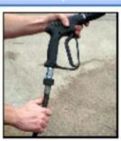
Attach trigger to high pressure hose.
