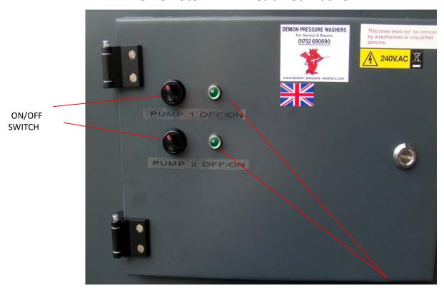
N.B. If there is no water in the machine a light will still indicate power but will not be operational. CHECK WATER
