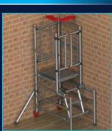
If you are positioning the LytePOD with the rear and side elevation against a surface/wall or are applying a lateral force from the back or side of the podium, position stabiliser at a 90 degree angle which is perpendicular to the podium. Fully tighten up the clamp on the stabiliser and ensure its secure.
