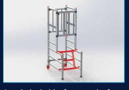
Attach the ladder frame to the front of the podium ensuring that all of the brace claws are locked into position. The ladder can be used to help square the podium.
