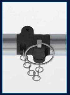
Once the podium has been unfolded, locate and lock in the bottom and top pins on the horizontal bracing at the back of the podium as shown in the diagram. If the top pin is inaccessible from the ground, lock in the top pin when the podium is fully assembled and accessed for the first time. There is no safety risk when doing this as the deck, ladder frame and bottom pin keeps the podium secure and free from any movement.
