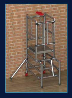
If you are positioning the LytePOD with the rear elevation against a surface/wall or are applying a lateral force from the back of the podium, position both stabilisers at a 90 degree angle which is perpendicular to the podium. Fully tighten up the clamps on each stabiliser and ensure both are secure.
