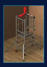
When the LytePOD is situated in an open area and work is being carried out overhead or from the rear of the podium, position the stabilisers at a 45 degree angle as shown in the image.
