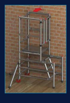
If you are positioning the LytePOD with a side elevation against a surface/wall or are applying a lateral force from the side of the podium, position one stabiliser at a 90 degree angle which is perpendicular to the podium and the other stabiliser parallel to the surface/wall. Fully tighten up the clamps on each stabiliser and ensure both are secure.
